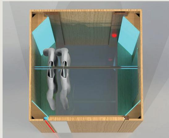
In case the door is locked from the outside and someone is still in the changing room, a motion sensor and a manual emergency shutdown is integrated, which stops the UV-C radiation for safety reasons.
